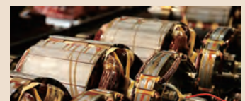
Varnishing of rotors for protection against vibrations, corrosion and harmful substances
